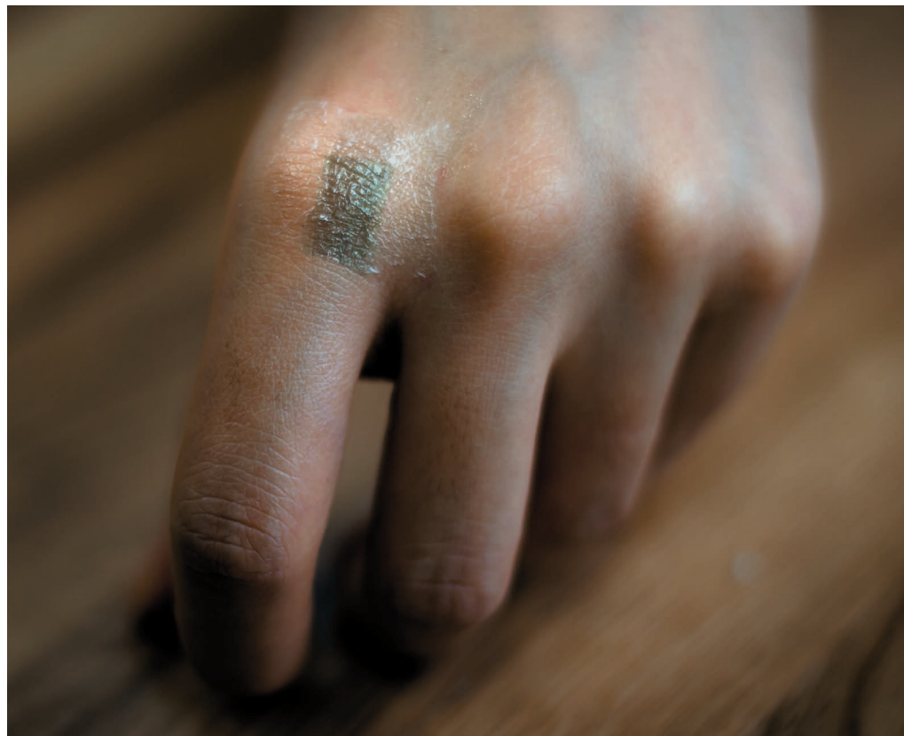
Unobtrusive ‘elastronic’ transistors can behave like skin and stretch without tearing.
